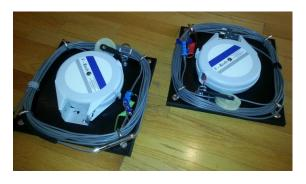
down the strip. They work in a similar way as a "bungee" type system; however, the bungee has been replaced by a pulley on a retractable cord. This makes the system considerably easier to set up, and the design of the reel platform also includes storage for the fencer's cables when they are not in use.
