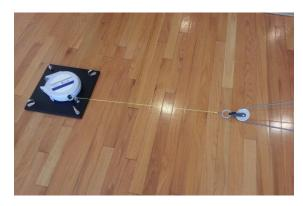
Viewed from end-of-strip: Pulling the fencer's connector forward causes the pulley to move forward, unwinding the reel against its spring. Retreating backward, the pulley takes up the cable slack as the reel's spring tension retracts the pulley.
