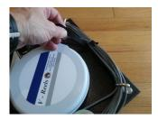
**Step 3:** Release the Velcro cable tie securing the loose end of the plug. Unwind the cable from the storage hooks.
