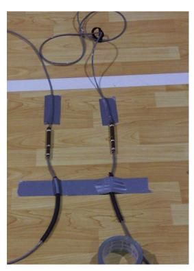
**Step 7:** At the center of the strip, tape down the cables as shown. Each cable is taped down over the rubber-reinforced section of the cable. This is the section of cable that will flex and the rubber hose provides additional strain relief.
