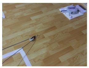
Viewed from end-of-strip: Pulling the fencer's connector forward causes the pulley to move forward, unwinding the reel against its spring. Retreating backward, the pulley takes up the cable slack as the reel's spring tension retracts the pulley.
