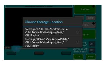
If you have both an SD card and a useable USB drive you will be able to choose which one to use during recording for the "copy to SD" destination. To choose the drive, turn the "copy to SD" option off and then back on:
